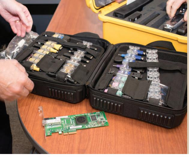
Pictured is a Cellebrite mobile device acquisition adapter kit. Digital forensic examiners must maintain a variety of adapters to ensure access to electronically stored information, wherever it is found.
